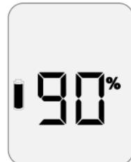
The device then displays the software version installed and remaining battery life. We recommend that you replace the battery as soon as it drops below 50%. Holding down the marking button in transmit mode will allow you to check battery life left at any time.
